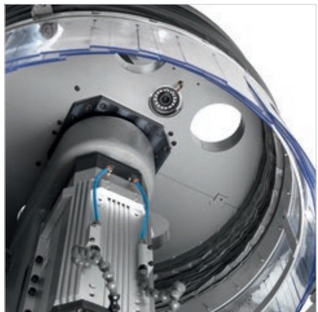
Position reading system with a video camera for centring large panels thanks to a rototranslation cycle in the machining program.
